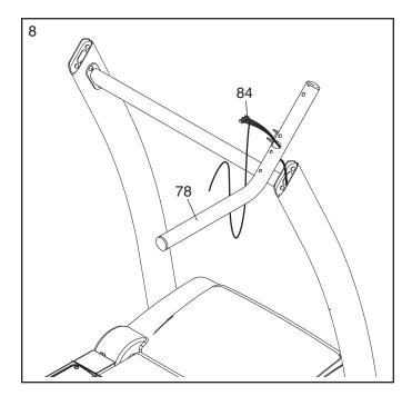
Attach the Handrails (77, 78) to the Uprights (81, 83) with four 5/16" x 2 1/2" Patch Bolts (5) and four 5/16" Star Washers (11).
